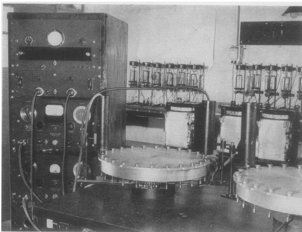
FIG. 5. APPARATUS FOR MEASURING THE RADIOACTIVITY OF \text{Fe}^{55} AND \text{Fe}^{59} SAMPLES
